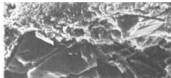
Figure 1B. The top one-fourth of this scanning electron micrograph shows the surface of the crust; beneath this is the entire thickness of the crust, followed by the calcite grains of marble, which is unaltered but has gypsum in the intergranular space
