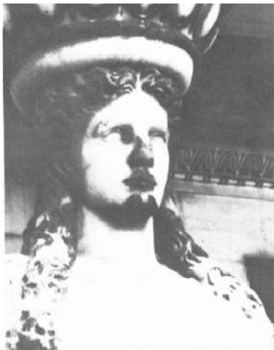
Figure 1A. The black crust, made of gypsum and soot, occurs in areas protected from rain. A portion of the crust is exfoliated at the site of the braids, obliterating details of the sculpture (Field Museum of Natural History, Chicago)
